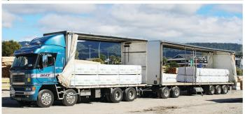
TC Transcontinental Packaging has been a leading supplier of wrap to the timber industry for over 40 years. In the last 12 months TC Transcontinental Packaging has developed the Renew<sup>TM</sup> timber wrap blend, a new blend containing a minimum of 30% recycled LDPE waste content by net volume. The product was developed with, and extensively trialled by Pukepine Sawmills.
